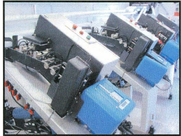
Fig 3-AutoFish System marking equipment
