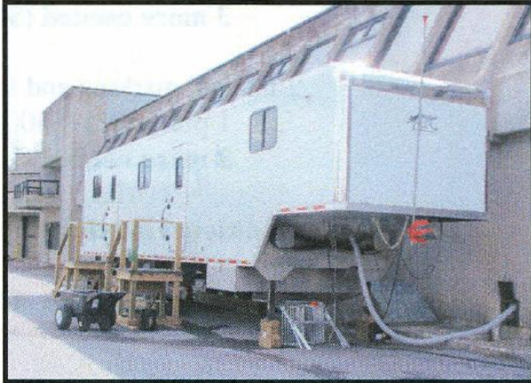
Fig. 1-Automated fish marking trailer (AutoFish System)
